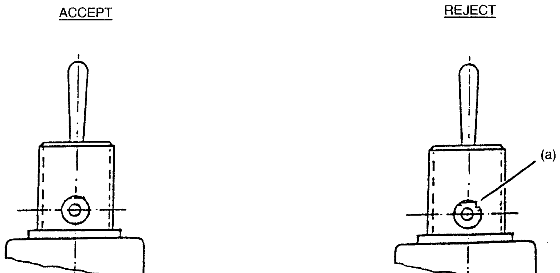
FIGURE II - CRACKS IN THE RIVET JOINT OF LEVER AXLE
