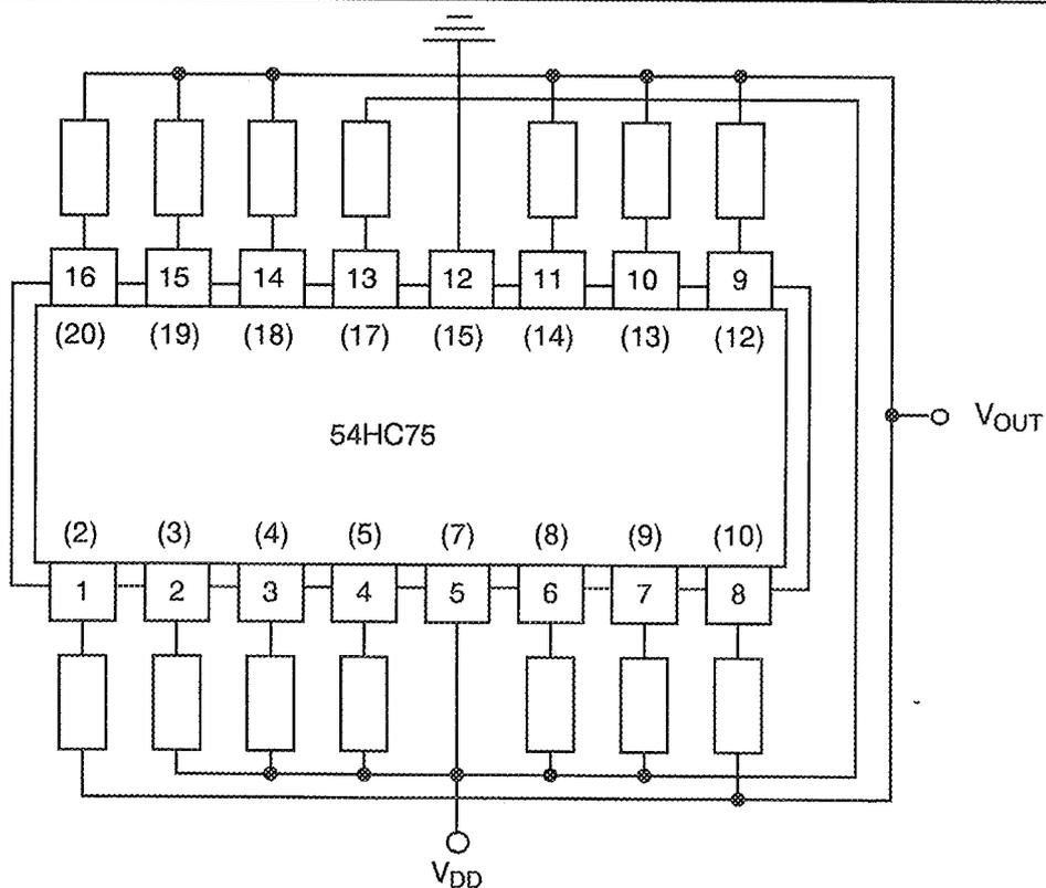
NOTES 1. Pin numbers in parenthesis are for the chip carrier package.
