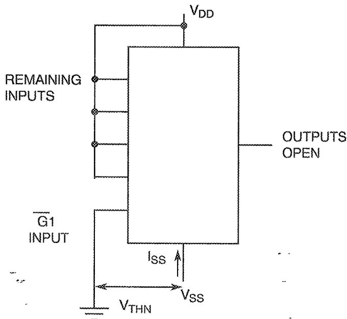
**FIGURE 4(g) - THRESHOLD VOLTAGE P-CHANNEL**
