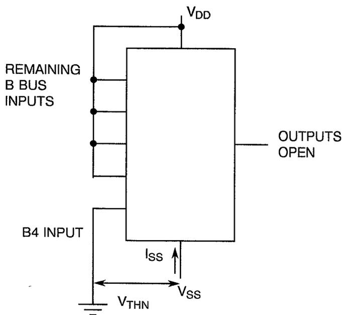
**FIGURE 4(g) - THRESHOLD VOLTAGE P-CHANNEL**
