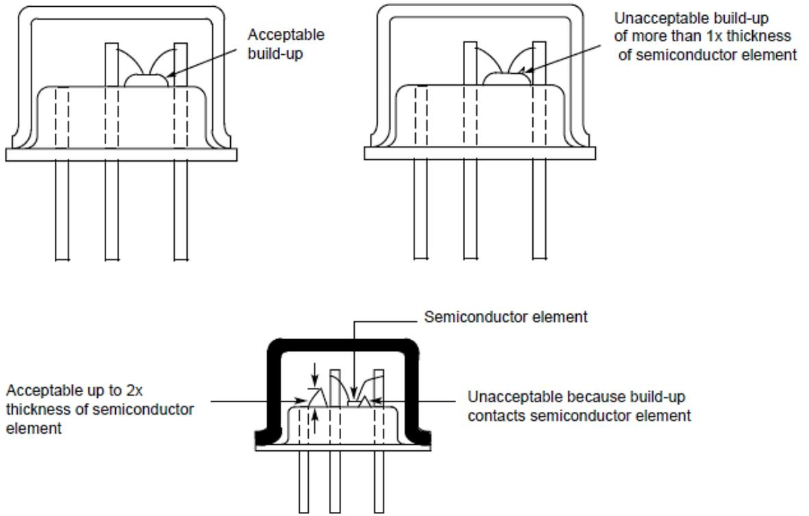
5.3 FIGURE 3: EXTRANEEOUS BONDING MATERIAL BUILD-UP
