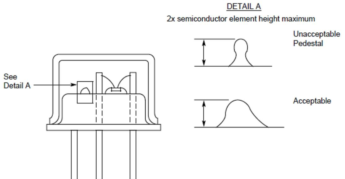
5.4 FIGURE 4: CLEARANCE IN DUAL-IN-LINE OR FLAT PACK TYPE DEVICE
