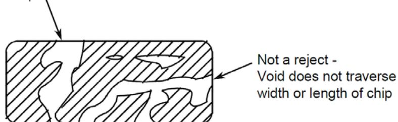
5.2 FIGURE 2: ACCEPTABLE AND UNACCEPTABLE BONDING MATERIAL BUILD-UP
