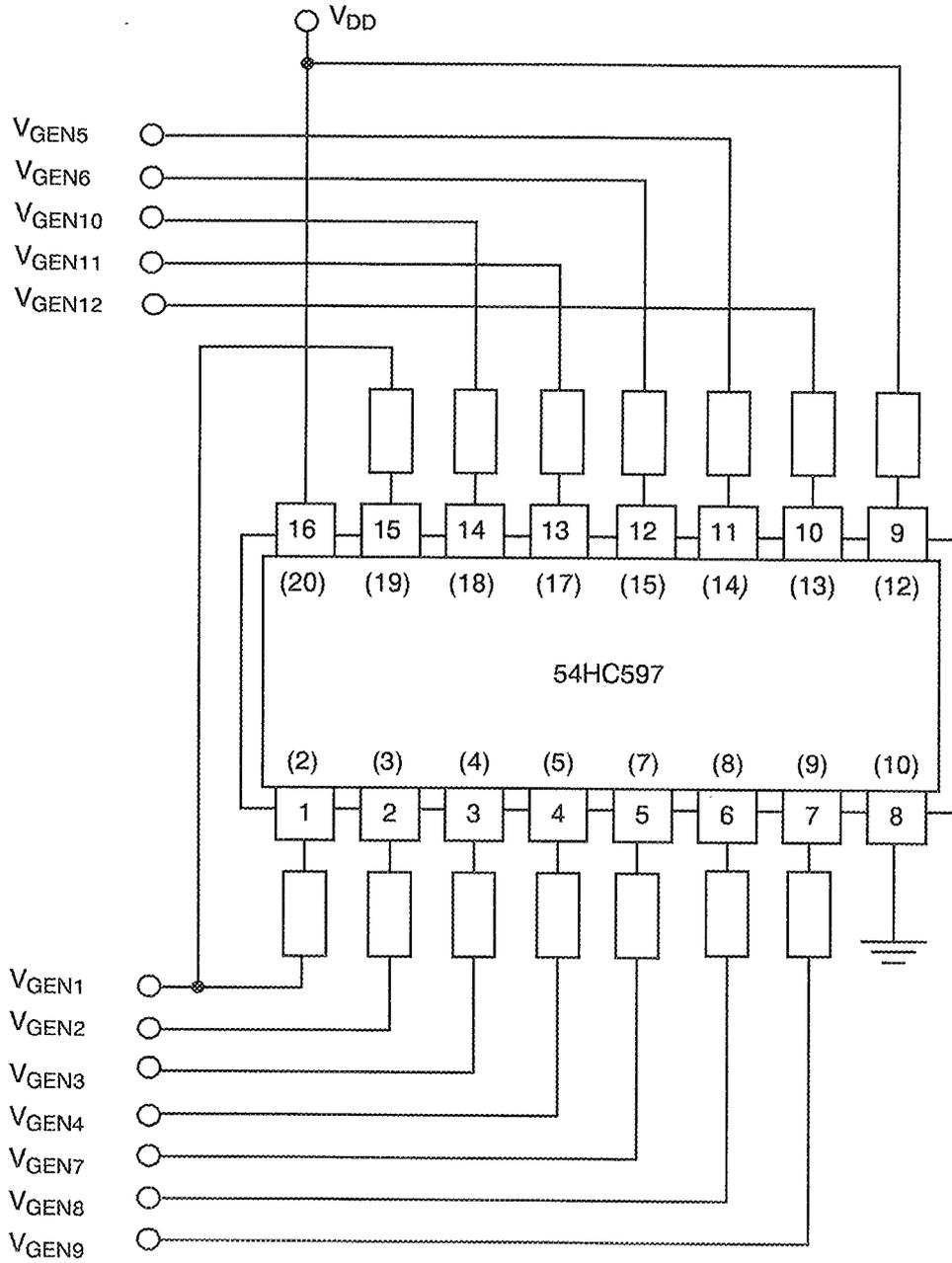
**NOTES** 1. Pin numbers in parenthesis are for the chip carrier package.
