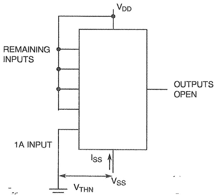
**FIGURE 4(g) - THRESHOLD VOLTAGE P-CHANNEL**
