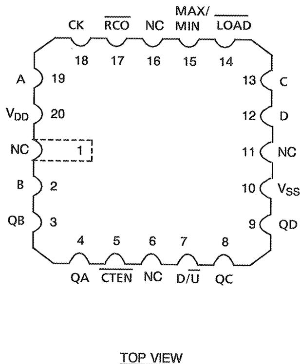
FLAT PACKAGE, SO AND DUAL-IN-LINE TO CHIP CARRIER PIN ASSIGNMENT
