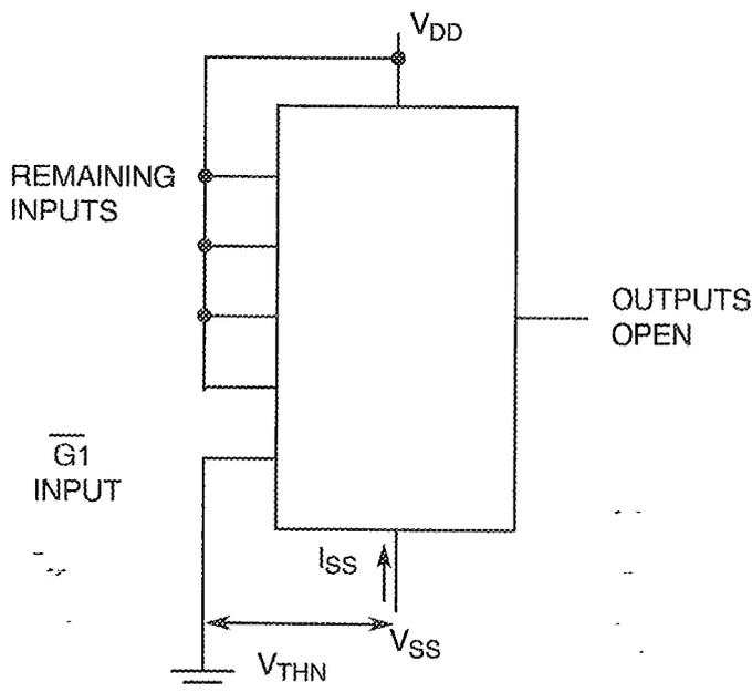
**FIGURE 4(g) - THRESHOLD VOLTAGE P-CHANNEL**
