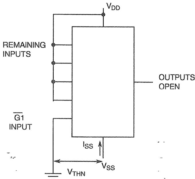
**FIGURE 4(g) - THRESHOLD VOLTAGE P-CHANNEL**
