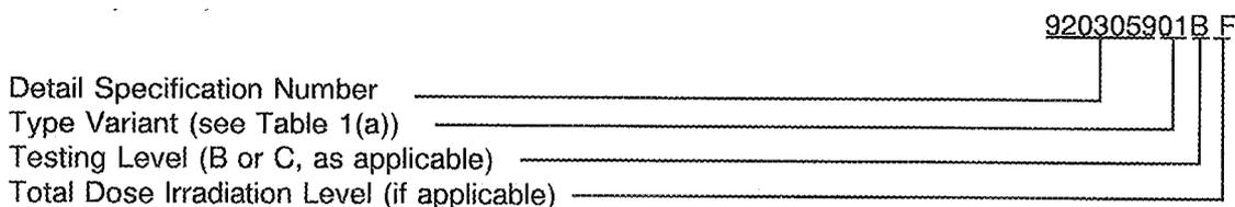
The Total Dose Irradiation Level designation shall be added for those devices for which a sample has been successfully tested to the level in question. For these devices, a code letter shall be added in accordance with the requirements of ESA/SCC Basic Specification No. 22900.
