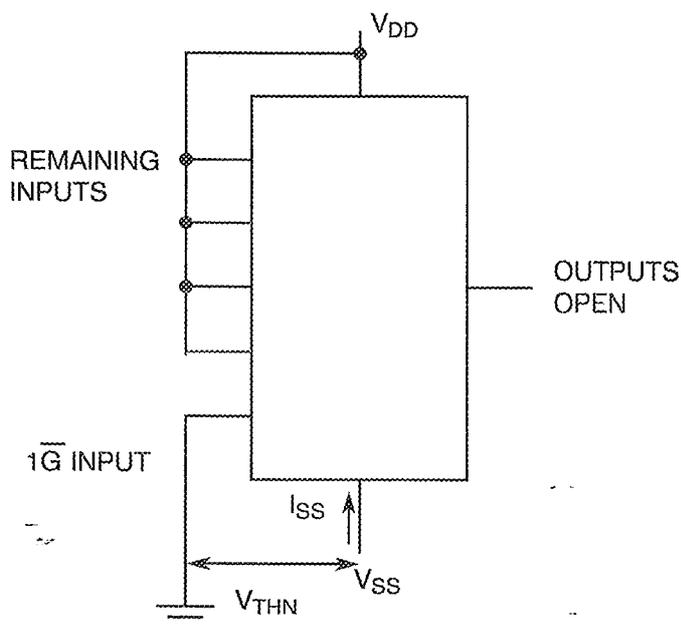
**FIGURE 4(g) - THRESHOLD VOLTAGE P-CHANNEL**
