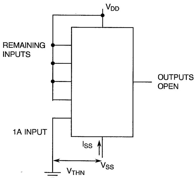
**FIGURE 4(g) - THRESHOLD VOLTAGE P-CHANNEL**
