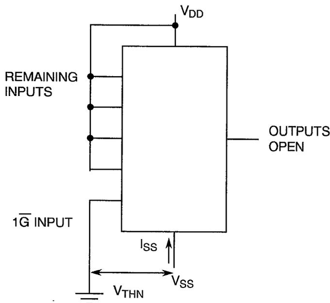
**FIGURE 4(g) - THRESHOLD VOLTAGE P-CHANNEL**
