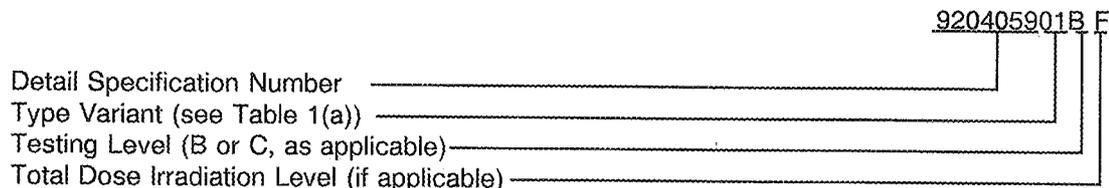
The Total Dose Irradiation Level designation shall be added for those devices for which a sample has been successfully tested to the level in question. For these devices, a code letter shall be added in accordance with the requirements of ESA/SCC Basic Specification No. 22900.
