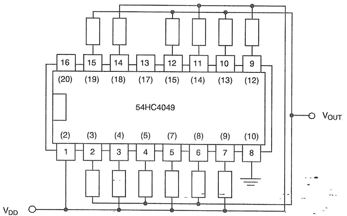
**NOTES** 1. Pin numbers in parenthesis are for the chip carrier package.
