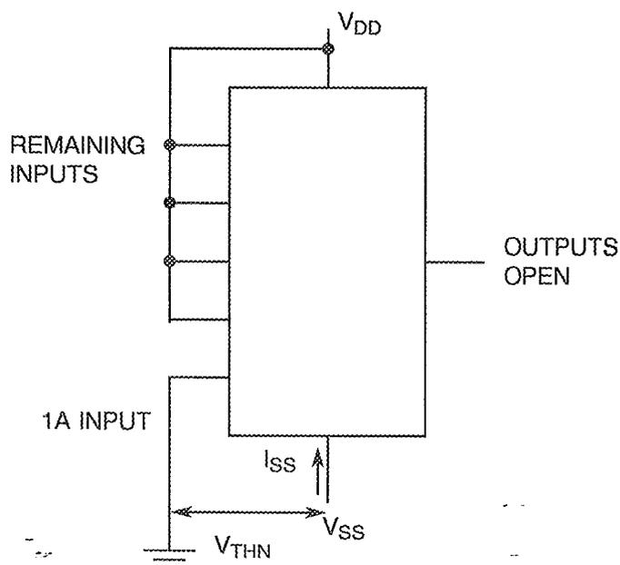
**FIGURE 4(g) - THRESHOLD VOLTAGE P-CHANNEL**
