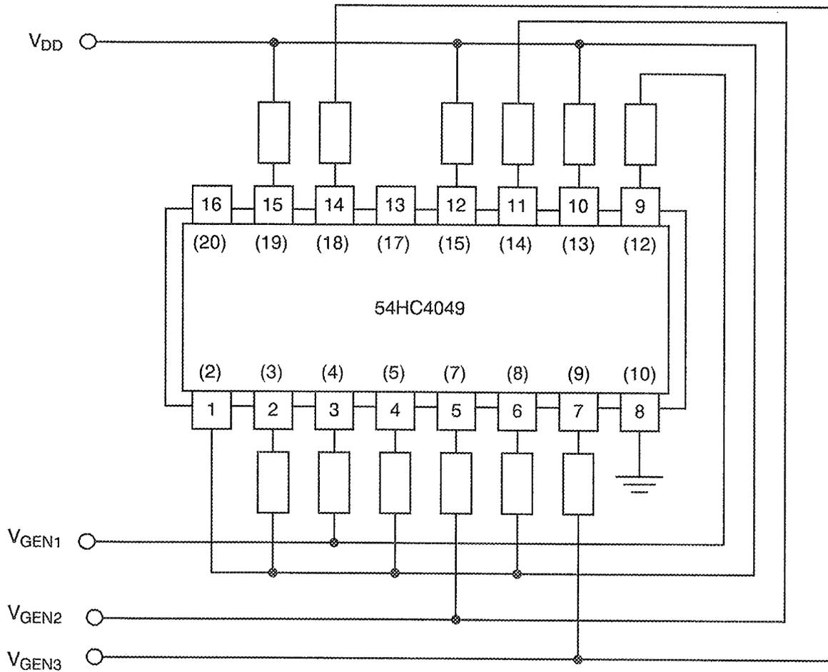
**NOTES** 1. Pin numbers in parenthesis are for the chip carrier package.
