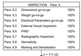
**INITIAL MEASUREMENTS** 100% Read and Record Room, High and Low Temperatures Electrical Measurements acc. ESCC Detail Specification
