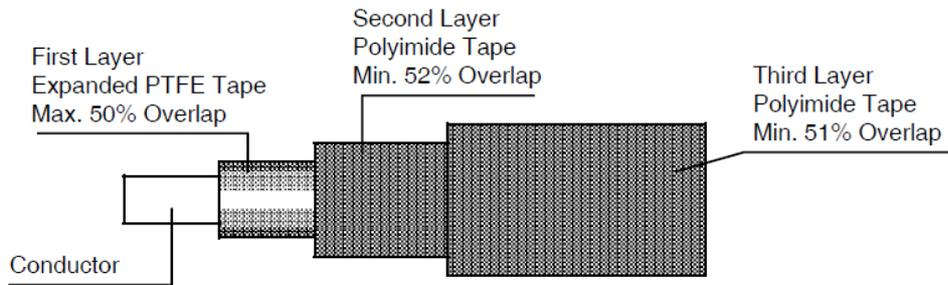
**FIGURE 2(b) – SINGLE CABLE WITH SHIELD AND JACKET**
