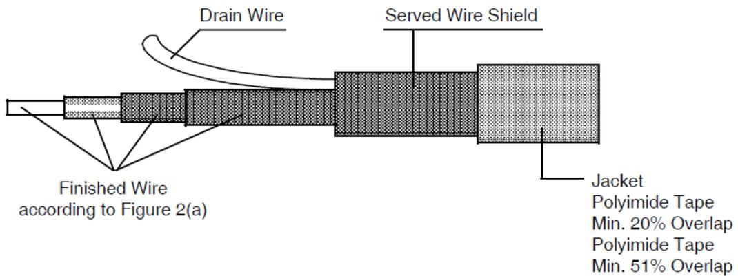
**FIGURE 2(c) – MULTICORE CABLE WITH SHIELD AND JACKET**
