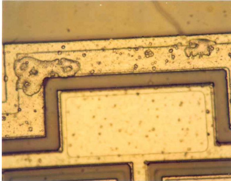
Figure 2 Evidence of Metallisation Blistering
