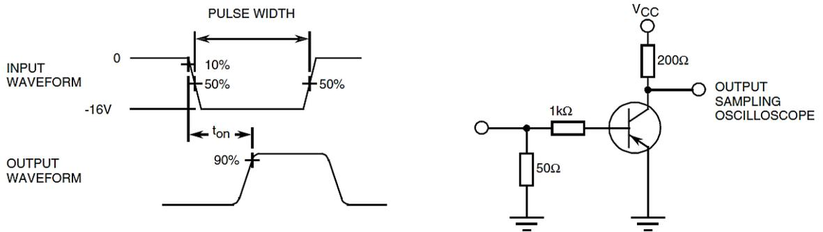
4.  $t_{off}$  shall be measured using the following test circuit. The input waveform shall be supplied by a pulse generator with the following characteristics:  $Z_{OUT} = 50\Omega$ ,  $t_r \leq 2ns$ , Pulse Width = 10 to  $100\mu s$ , Duty Cycle  $\leq 2\%$ . The output waveform shall be monitored on an oscilloscope with the following characteristics:  $Z_{IN} \geq 100k\Omega$ , input capacitance  $\leq 12pF$ ,  $t_r \leq 5ns$ .
