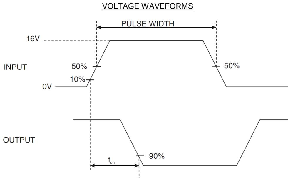
4.  $t_{off}$  shall be measured using the following test circuit. The input waveform shall be supplied by a pulse generator with the following characteristics:  $Z_{OUT} = 50\Omega$ ,  $t_r \leq 2ns$ , Pulse Width =  $10\mu s$ , Duty Cycle  $\leq 2\%$ . The output waveform shall be monitored on an oscilloscope with the following characteristics:  $Z_{IN} \geq 100k\Omega$ , input capacitance  $\leq 12pF$ ,  $t_r \leq 5ns$ .
