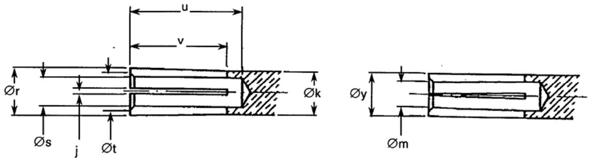
**FIGURE 3 – STANDARD TEST CONNECTOR INTERFACE – FEMALE CONTACT
