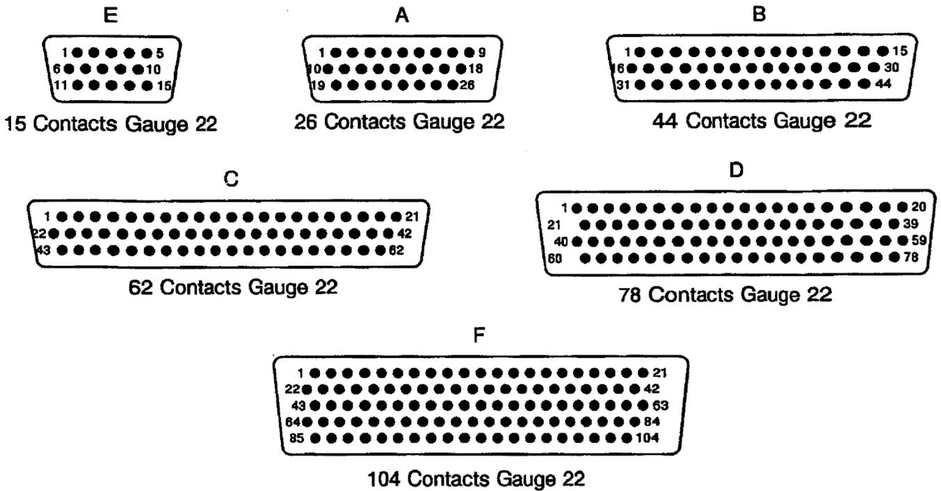
POWER AND COAXIAL CONTACT ARRANGEMENTS (VARIANT 01)
