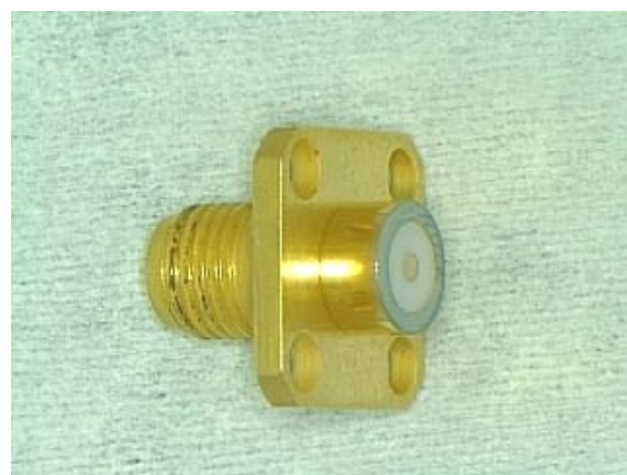
After mechanical rework of the back face
