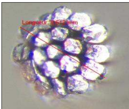
Wire conductor diameter : 0,61 mm
