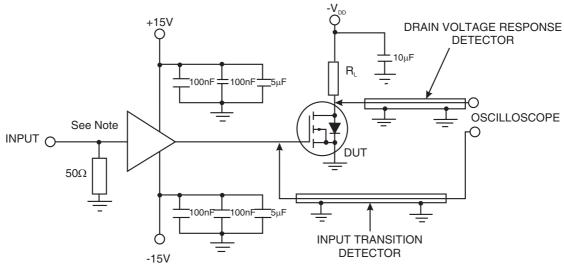
**NOTE:** The amplifier shall be a suitable voltage follower/buffer amplifier. <u>VOLTAGE WAVEFORMS</u>
