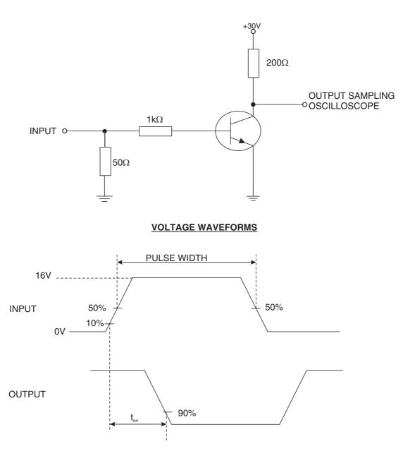
4.  $t_{off}$  shall be measured using the following test circuit. The input waveform shall be supplied by a pulse generator with the following characteristics:  $Z_{OUT} = 50\Omega$ ,  $t_r \le 2ns$ , Pulse Width = 10 to 100 $\mu$ s, Duty Cycle  $\le 2\%$ . The input and output waveforms shall be monitored on an oscilloscope with the following characteristics:  $Z_{IN} \ge 100k\Omega$ , input capacitance  $\le 12pF$ ,  $t_r \le 5ns$ .
